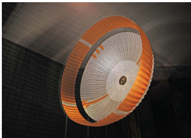
PARACHUTE TEST In April 2009 engineers tested the rover's parachute in the world's largest atmospheric wind tunnel, at NASA's Ames Research Center. The parachute is nearly 16 meters (52 feet) across. Most of the fabric is nylon.
