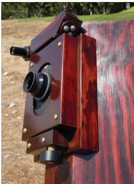
One of the Dob Buster's unusual features is the mirror-fed, right-angle finder, which attaches to the telescope tube with magnets. Another is the low-profile sled focuser. Both are described in the accompanying text.
