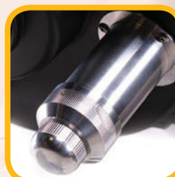
The f/8 optical system comes with an internal Crayford-style 7:1 focuser
