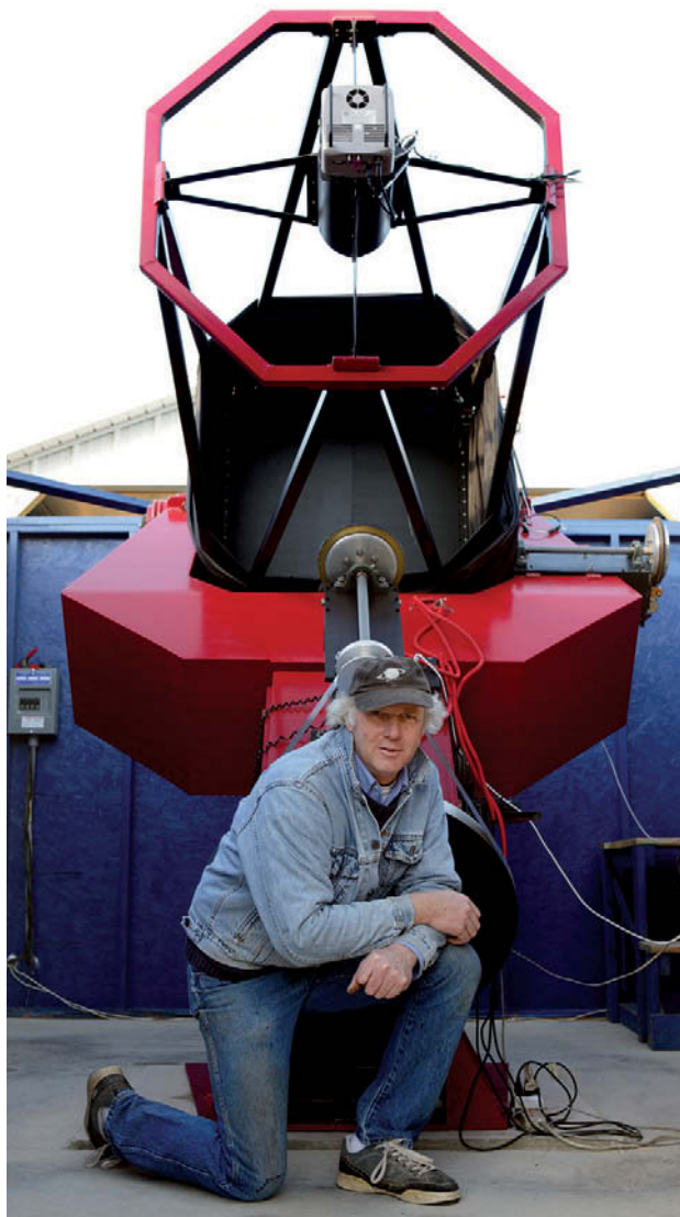
WORKHORSE Bob Holmes with his fork-mounted 32-inch telescope. All of his scopes have large CCD cameras permanently mounted at the focus; there's no place for an eyepiece.
