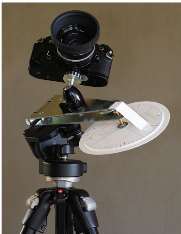
The hinge mount is assembled from a handful of common hardware-store items and requires no machining. In addition to the tracker, you'll need a photographic ball head and a regular camera tripod to complete the setup.
