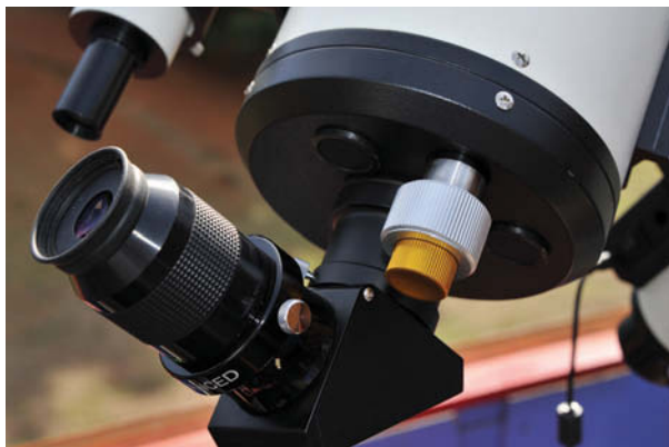
The MAK 150mm features a dual-speed focuser with a very light touch. In addition to offering precise focusing at high magnifications, an internal preload keeps images in the same position when reversing the direction of either focusing knob.
