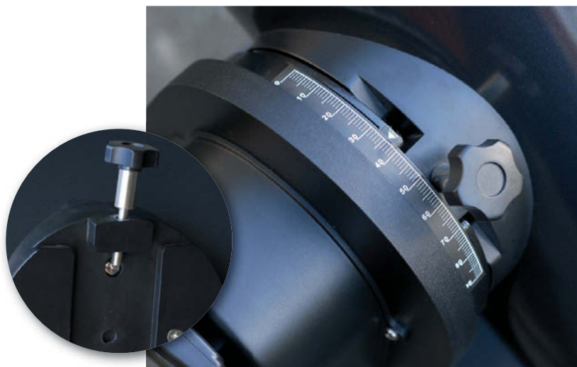
Left: The scope's focuser-side altitude trunnion engages a dove-tail fitting on the motor and bearing assembly attached to the base, and locks into position with a large, captive hand knob ( inset ). Loosening the hand knob allows you to quickly and easily separate the optical tube assembly from the mount for transport and storage. Right: A silky smooth 2-inch focuser is standard equipment with the XT10g. The focuser features a 10:1 reduction mechanism for ultra-precise fine focus. The red-dot finder is familiar equipment to most readers.
