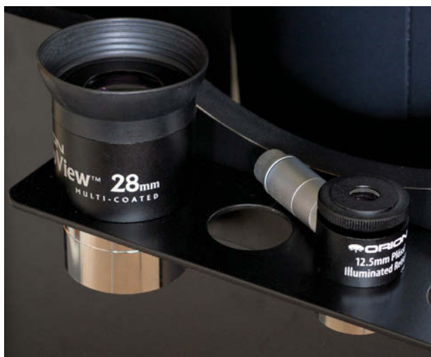
The scope includes two eyepieces: a 28-mm for wide-field viewing and locating objects, and a 12.5-mm illuminated reticule Plössl to aid in centering alignment stars. A handy eyepiece rack attaches to the front of the rocker box.
