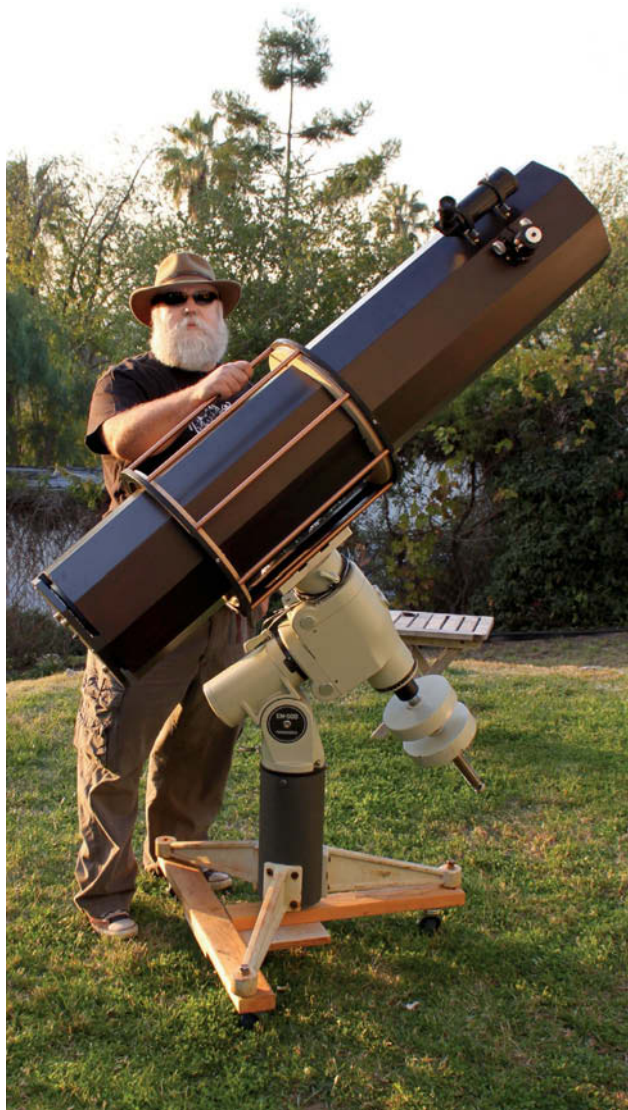
Parker poses with his newly completed 10-inch f/6 Newtonian, featuring a beautifully finished wooden tube. The scope rides on a Takahashi equatorial mount and utilizes a rotating ring assembly that he built himself.
