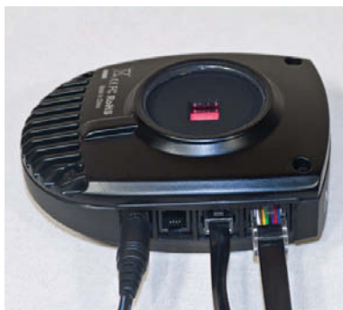
Left: While the NexGuide can be screwed directly onto any adapter having standard T threads, it's best to use the included 1¼-inch nosepiece as this will allow you to easily swap the NexGuide for an eyepiece. Right: The NexGuide requires three cable connections for power, the guiding cable, and the hand controller.
