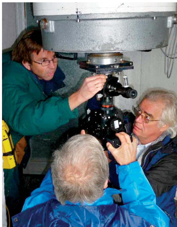
MOMENT OF TRUTH Johan Knapen (left), Berthold Stober (right), and John Morrison attach the team's custom-built spectrograph and guiding-eyepiece assembly to the telescope.
