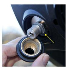
The well-designed mirror locks have a pin (arrowed) that presses on a wire rod (attached to the mirror support) when a conical sleeve in the hand knob is tightened. This allows the locks to be engaged without upsetting the scope's focus.
