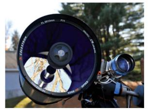
As detailed in the text, Celestron's camera adapter (*far left*) is based on the photographic T system. Also explained in the text, the new EdgeHD optics have a removable secondary mirror, and they remain compatible with Starizona's HyperStar f/1.9 imaging system. The EdgeHD 14's long (3,910 mm) focal length is great for shooting galaxies. This full-frame view of M33 was made with a KAF-16803 CCD and, as with the Veil picture on page 52, a total exposure of 150 minutes through Astrodon filters.
