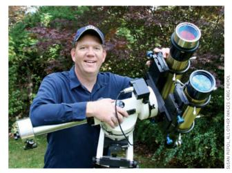
Maryland amateur astronomer Greg Piepol poses with two of his solar telescopes. The upper scope is a Coronado SolarMax 90  $H\alpha$  telescope, while the other is a similar model that passes the calcium K (CaK) line of the spectrum.
