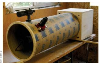
The author's scope rests on a hardwood dowel so that its horizontal balance point can be determined. The square tube section makes it easy to position side bearings at the balance points.
